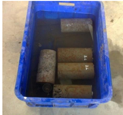
Gambar 4. Perendaman silinder beton
